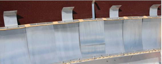
The HMT Secondary Wiper Seal is a proven secondary seal that has been protecting storage tanks in the AST industry for over 30 years. The Secondary Wiper Seal has exceptional gap sealing ability, long service life and a maintenance free operation. The HMT Secondary Wiper Seal is designed to accommodate wide rim space variations and will return to the tank without special attention if the tank is overfilled.
