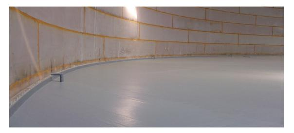
The DeckMaster GRP floating roof is a seamless, non-metallic full-contact floating roof. It's gastight polypropylene honeycomb core is "sandwiched" between multiple layers of fiberglass utilizing modern high-grade Vinyl Ester resins designed to be resistant to most hydrocarbons in the petrochemical industry. The result is a smooth, seamless and virtually indestructible full-contact floating roof that also is corrosion free, thus necessitating little or no maintenance.
